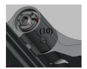
Open the door and loosen the M6x5 set screw  $\bigcirc$  (10).
